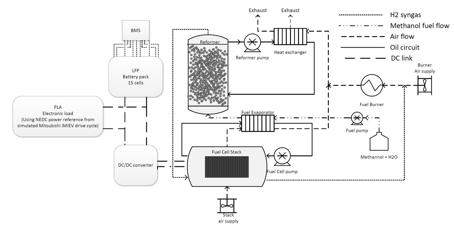
Fig. 1: Fuel cell range extender and battery pack.
